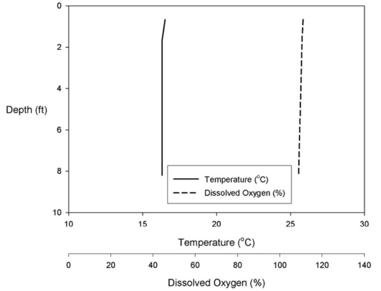
Figure 5-2. Dissolved oxygen saturation measurements from YSI 6600V2 sonde deployed at 7.1 ft at Santuit Pond deep spot
