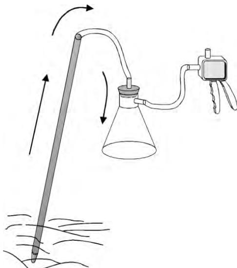
Littoral Interstitial Porewater Sampler
