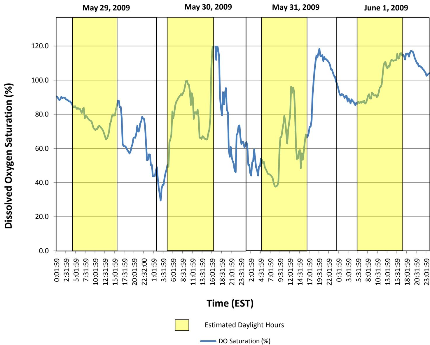
Figure 5-3. Dissolved oxygen saturation measurements from YSI 6600V2 sonde deployed at 7.1 ft at Santuit Pond deep spot and mean wind speed recorded at Otis Airforce Base
