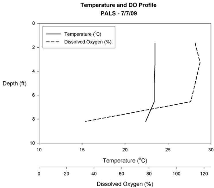
**Figure 5-1c. Temperature and Dissolved Oxygen Profiles for Santuit Pond**
