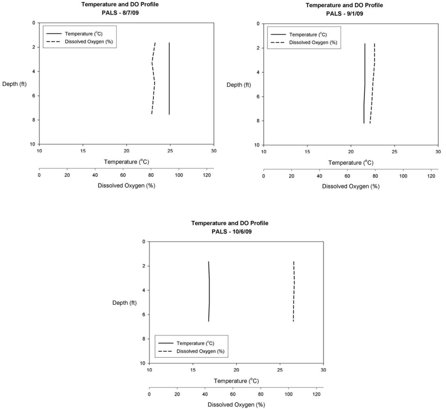
Figure 5-1d. Temperature and Dissolved Oxygen Profiles for Santuit Pond
