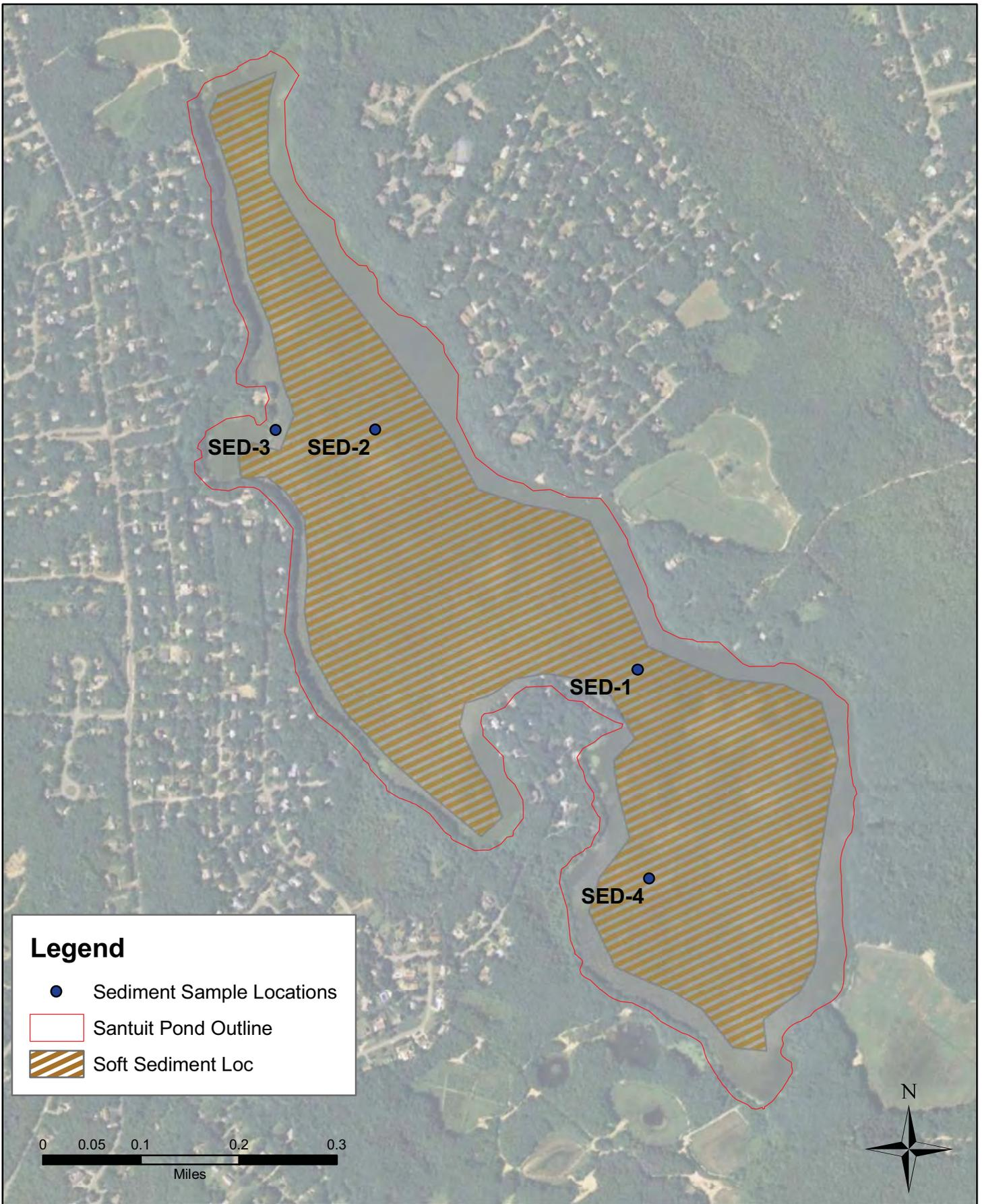
**Figure 3-5. Santuit Pond sediment sampling locations and soft sediment coverage**
