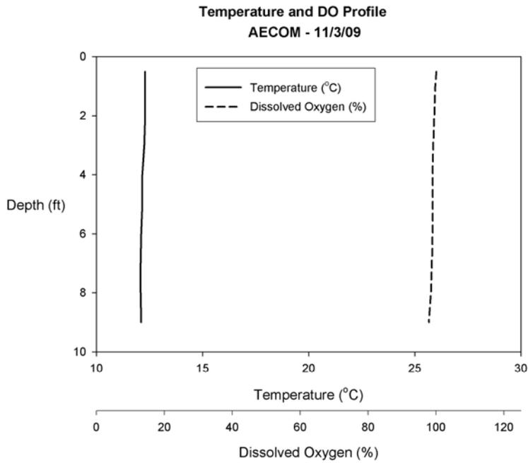
**Figure 5-1b. Temperature and Dissolved Oxygen Profiles for Santuit Pond**
