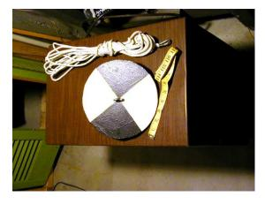
A Secchi disk is an 8-inch (20 cm) disk with alternating black and white quadrants. It is lowered into the water of a lake until it can be no longer seen by the observer. This depth of disappearance, called the Secchi depth, is a measure of the *transparency* of the water. The Secchi disk measures
