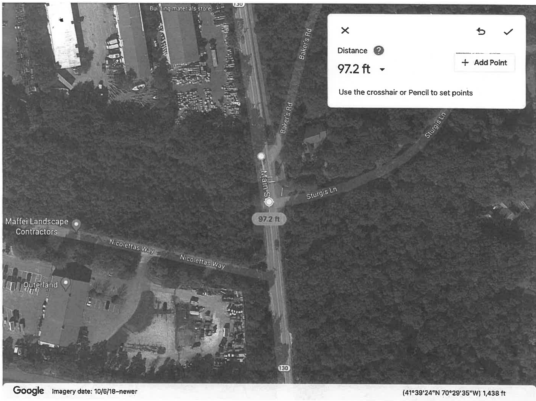
EXHIBIT B The distance from proposed curb cut to the intersection of Sturgis Lane is 97.2 feet. Far less than the 200-foot minimum. Also note the pedestrian and bike crossing between Sturgis Lane and Baker Road.
