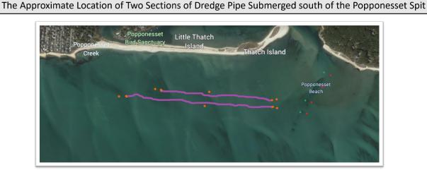
There is a total of ~4,800' feet of pipe in two sections (~3,200' & ~1,600') submerged in approximately 5' of water just south of the Popponesset Spit. There are Orange & White Poly Balls marking the location of the end of the pipe & anchor at each end. There is also a second Poly Ball marking the mid-points of each pipe.
