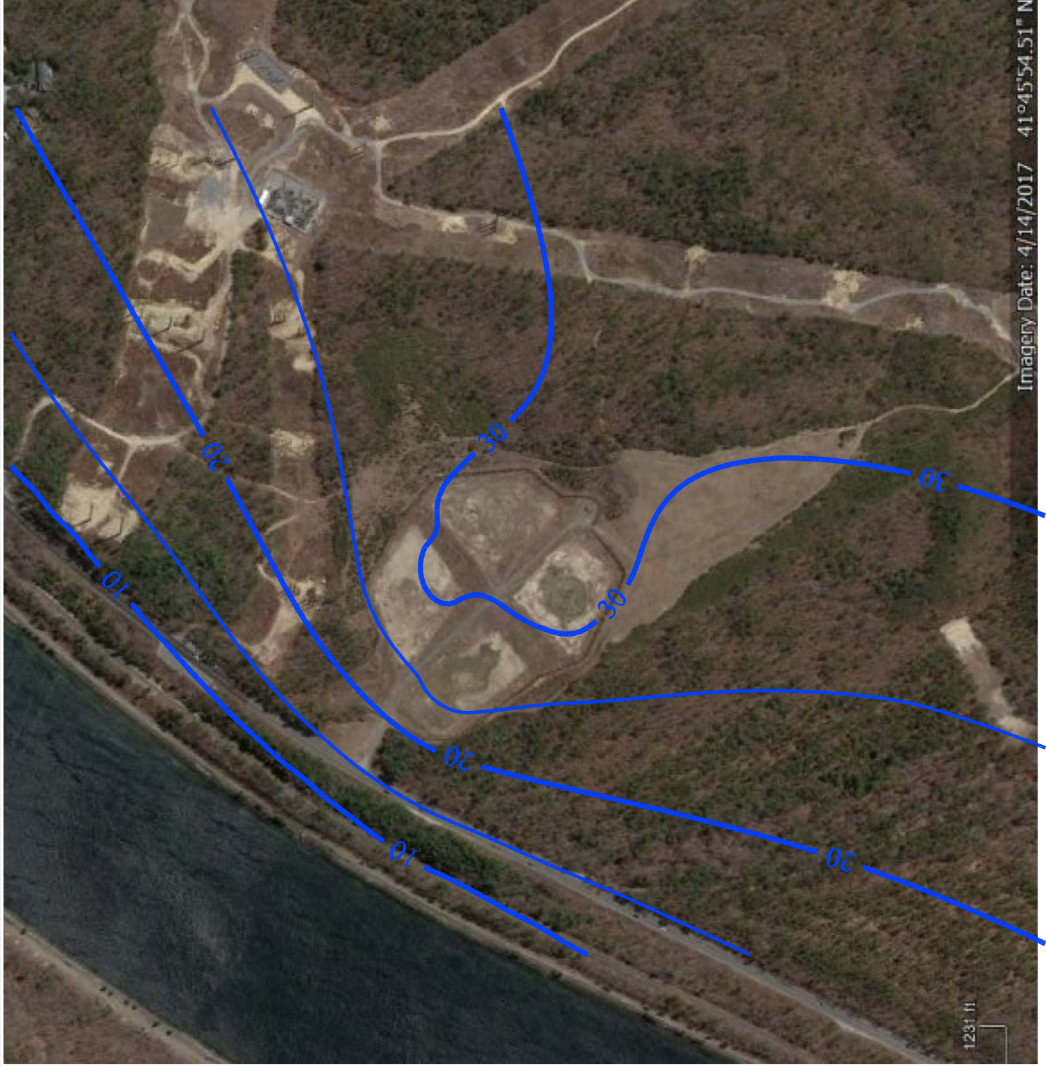
Figure 3. Simulated Groundwater Elevation Contours, Loading at 5 gpd/sf* or 1,295,800 gpd.
