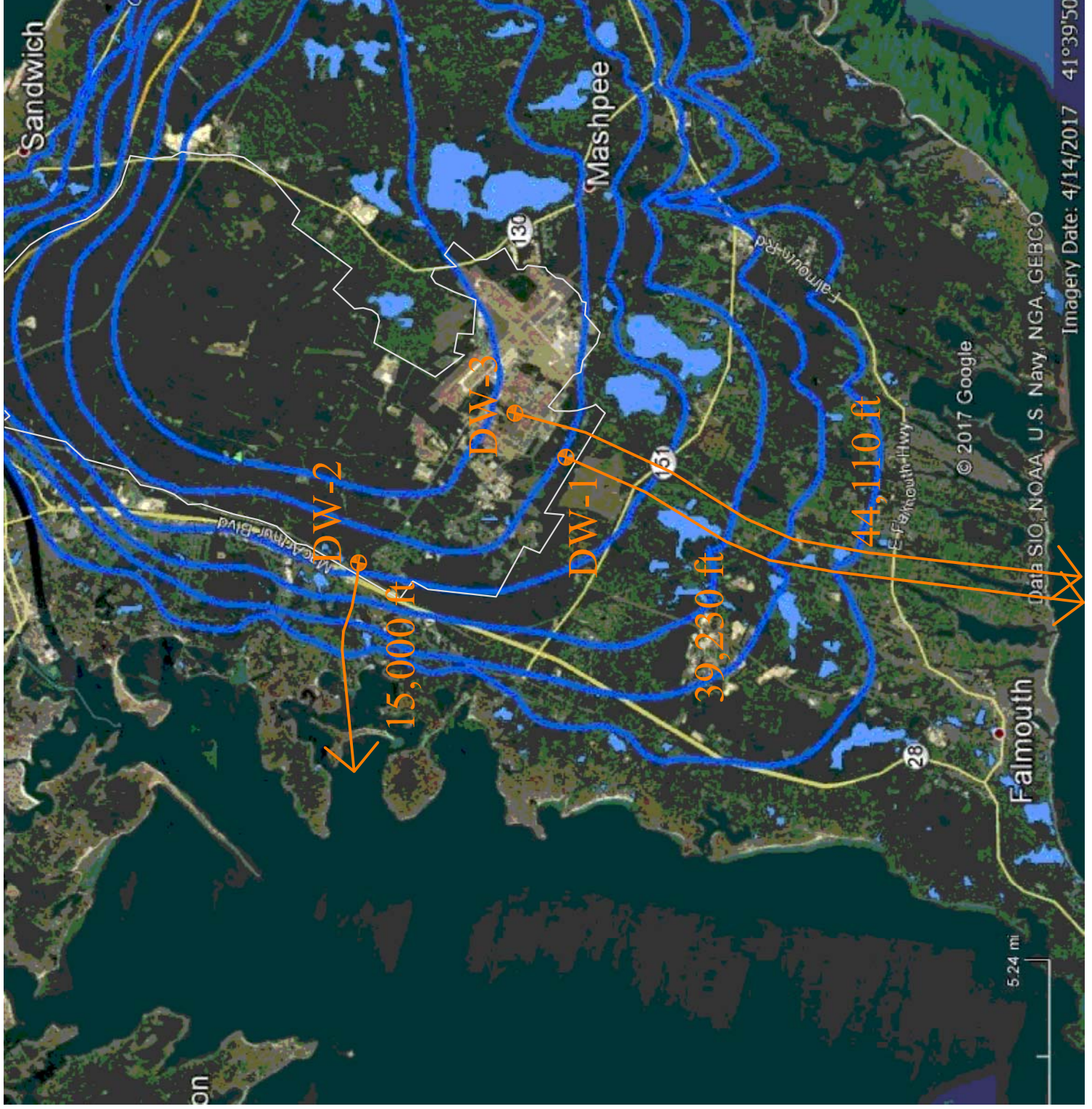
Figure 8. Groundwater Flow from Three Possible Deep Wells, DW-1, DW-2 and DW-3.
