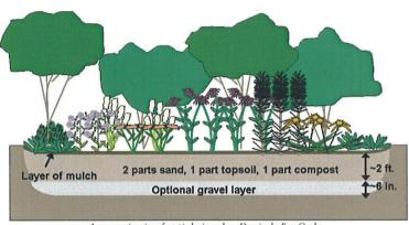
A cross-section view of a typical rain garden. Drawing by Sara Grady.
