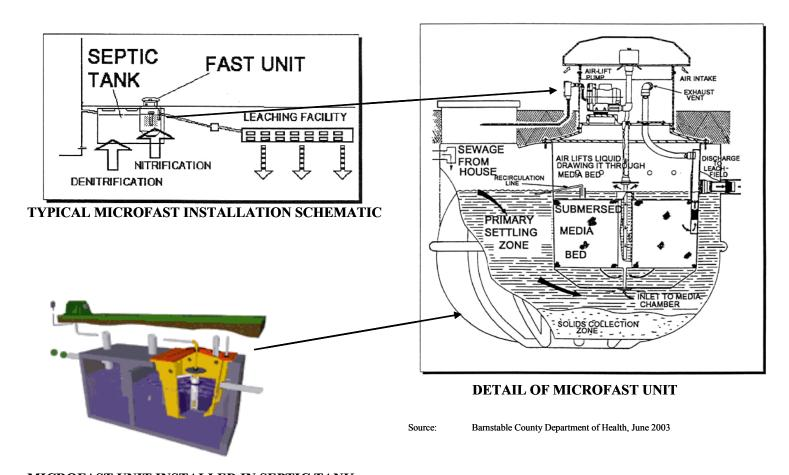
MICROFAST UNIT INSTALLED IN SEPTIC TANK
