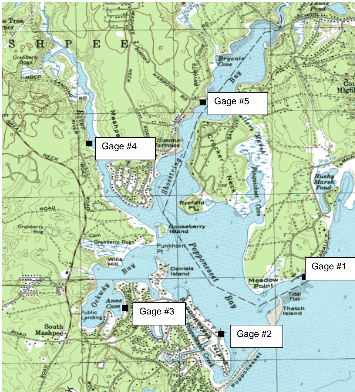
Figure V-6. Map of the study region identifying locations of the tide gauges used to measure water level variations throughout the system. Five (5) gauges were deployed for one month between October 4 and November 5, 1999. Each black square represents the approximate locations of the tide gauges (1) Offshore of the inlet to the northeast of Thatcher Island, (2) on the eastern shore of Popponesset Island, (3) within Anns Cove (Ockway Bay), (4) in the Mashpee River, and (5) on the western shore of Shoestring Bay.
