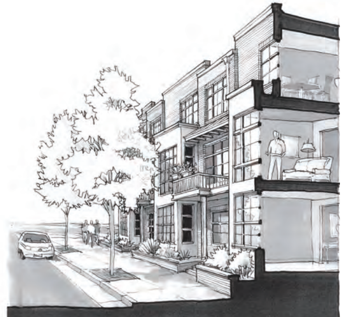
Figure 1.8: Section-perspective drawing of a three-story apartment building placed close to the sidewalk, creating an urban character that may be proper for certain parts of the neighborhood. From The Design Book: The Northern Neighborhoods , Stapleton.
