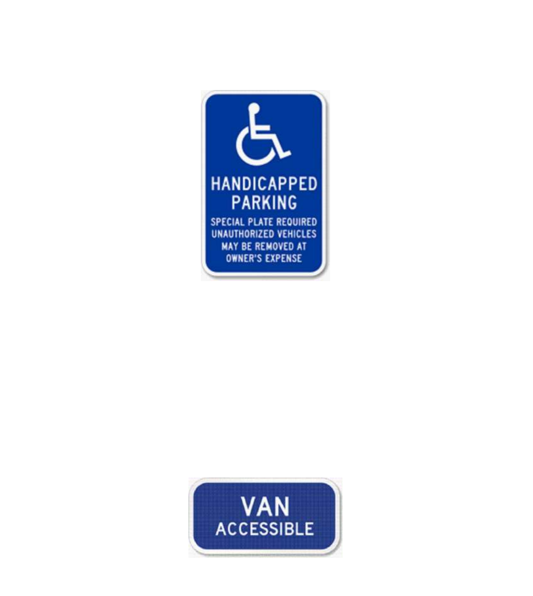
C-727 ACCESSIBLE PARKING SIGN DETAIL N.T.S.
