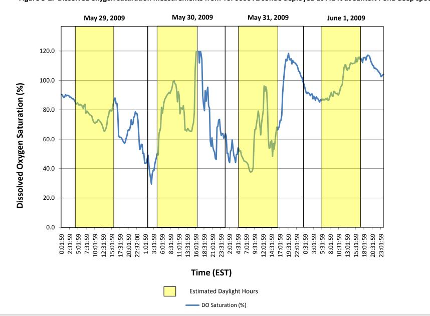
Figure 5-2. Dissolved oxygen saturation measurements from YSI 6600V2 sonde deployed at 7.1 ft at Santuit Pond deep spot
