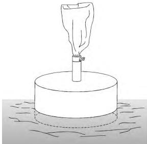
Littoral Interstitial Porewater Sampler
